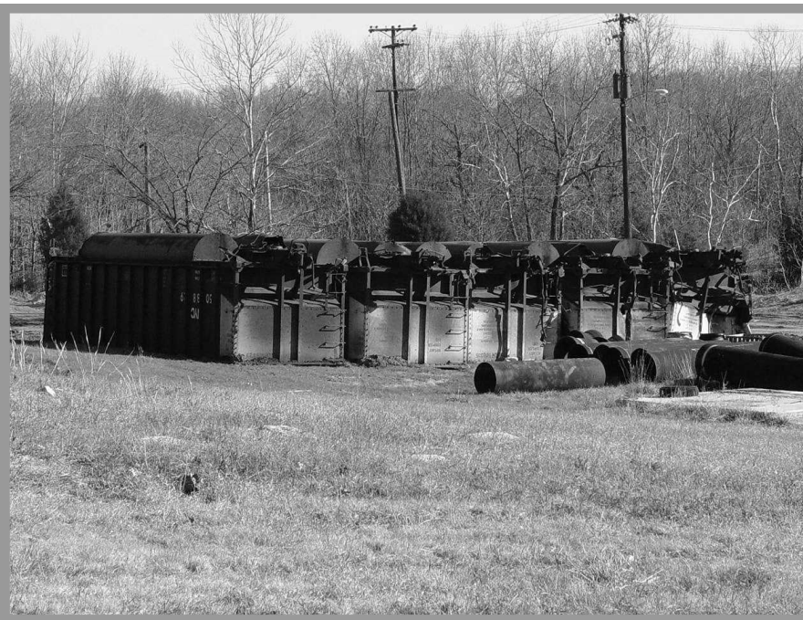
Remnants of the December 26th 22 car derailment at the north end of Latham siding on CSX's Henderson Sub are piled (less trucks) in the Rogers Materials quarry yard prior to scrapping. At least 20 of the 22 cars will be scrapped. Rail and switch repairs were on-going during January digital image Chuck
