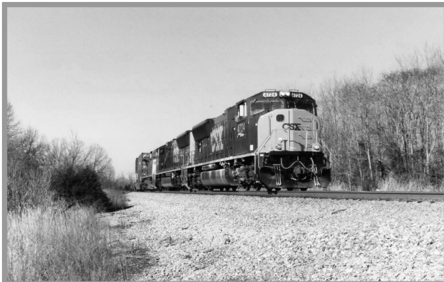
CSX is taking delivery of 20 EMD SD70MACs in early 2004. These units are in compliance with new emission regulations and sport the 'Bright Future' paint scheme. Here 4724 and 4726 and a C40-8W are pulling Q121 southbound at Crofton on January 10, 2004. from a color print by Wallace
